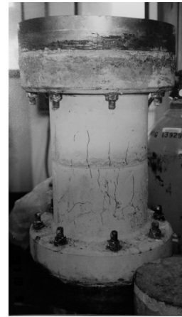
Photo 3 Crack pattern after testing under air dry and loading condition
