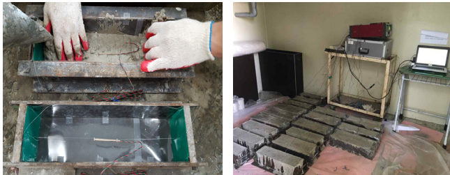
(a) Gauge installation (b) Test in humidity chamber
