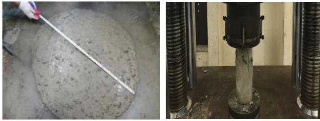
(a) Slump flow (b) compressive strength
