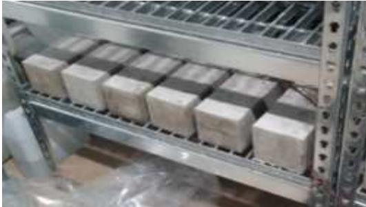
Figure 9. Drying shrinkage specimens
