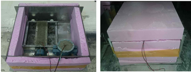
Photo 1. Installation of thermocouple and strain gauge with insulating curing method
