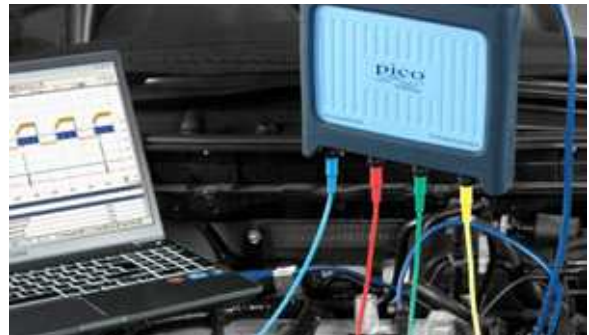
Fig. 2. Pico automotive diagnostics kit.
