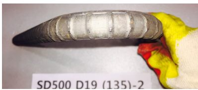
Fig. 3. Surface condition after bending test
