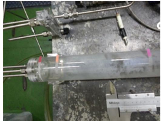
Fig. 5 Length measurement of recombination for ammonium carbamate in the acrylic tube
