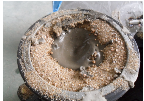
Fig. 9. Compaction effect test using mold
