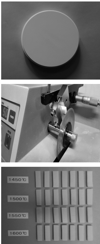
Figure 2. Zirconia block cutting with diamond wheel.
