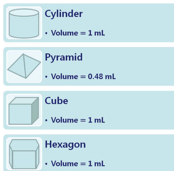
Fig. 1. Four geometric objects with predefined dimensions made of Teflon-perfluoroalkoxy material were fabricated using a highly precise computer numerical-control milling machine. The volumes of the cylinder, pyramid, cube, and hexagon blocks ranged between 0.48 mL and 1 mL.
