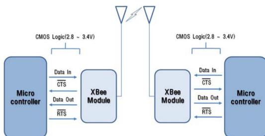
Fig. 4. Configuration of XBee Module Communication.
