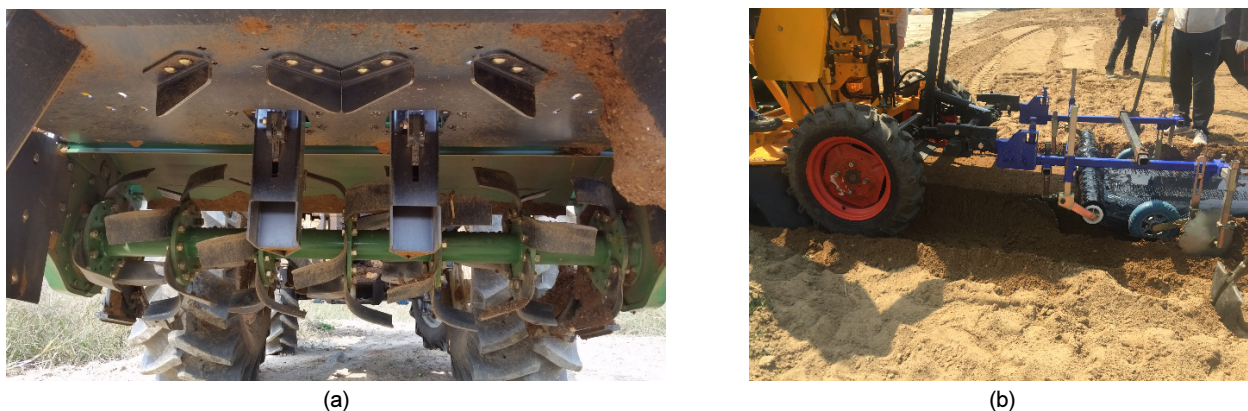
Figure 3. The rotavator and digging device for soil cutting (a) and soil covering device after seeding process (b).
