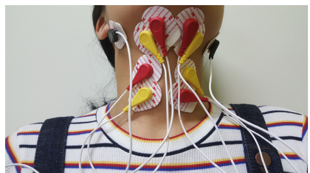
Figure 3. Attachment of EMG Electrode
