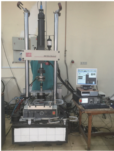
Fig. 2. View of the Mini Bionix II device in which the insertion - separation cycles were performed.
