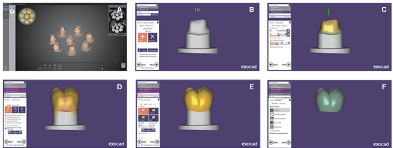
Fig. 2. Interim crown design. (A) Multi die scan, (B) Margin set-up, (C) Cement space set-up, (D) Tooth placement, (E) Margin modification, (F) Merge and save restoration.
