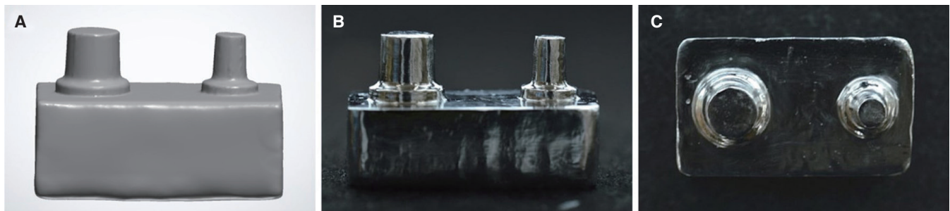
Fig. 2. Preparation of the master model. (A) STL file of the master model, (B) Front view of the fabricated alloy master model, (C) Occlusal view of the fabricated alloy master model.
