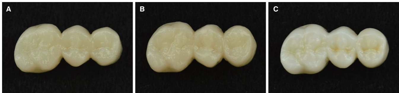
Fig. 3. Fabrication of three-unit FDPs. (A) LZ group: lithium disilicate glass ceramics pressed on zirconia-based FDPs, (B) ML group: monolithic lithium disilicate FDPs, (C) MZ group: monolithic zirconia FDPs.
