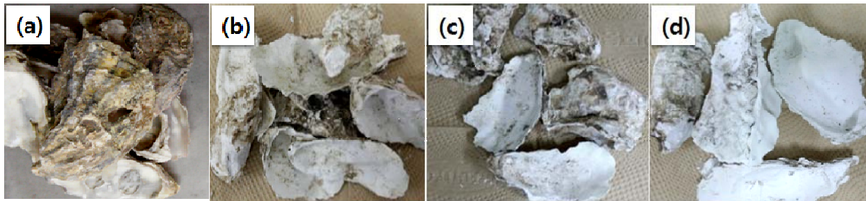
Fig. 4. Oyster shell waste calcination at different temperatures (a) Before calcination, (b) Calcination at 900 oC, (c) Calcination at 1000 oC and (d) Calcination at 1200 oC.
