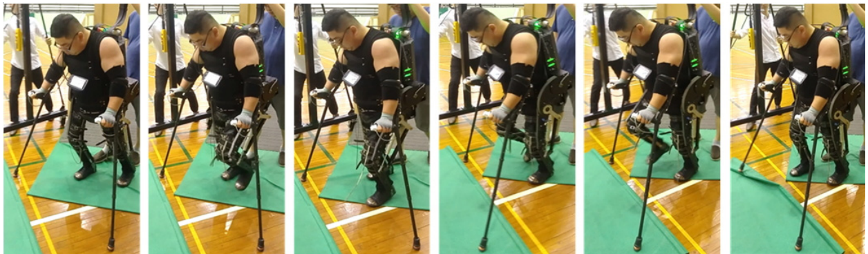
Fig. 5. The forward inflection walking with WalkON Suit
