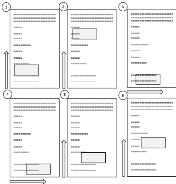
Fig. 8 Procedures of BLF(Bottom-Left-Fill) algorithm
