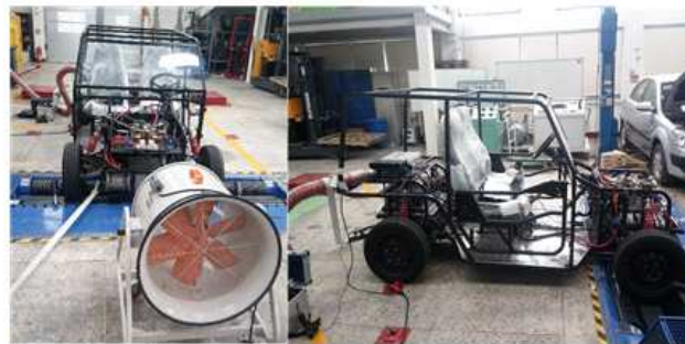
Fig. 19. Maximum power/speed test using dynamo meter.
