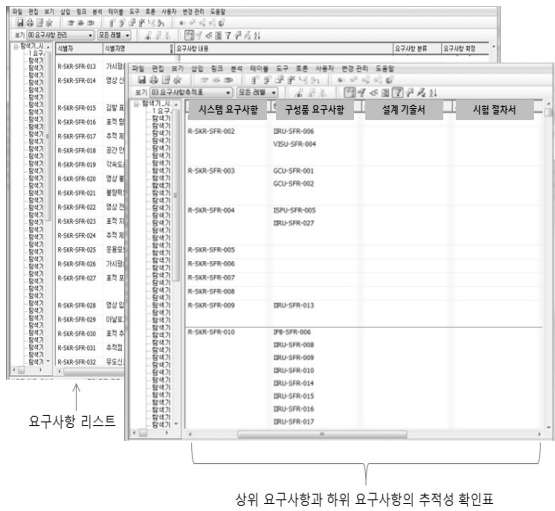
[Figure 10] Requirements and Tracking Matrix in DOORS
