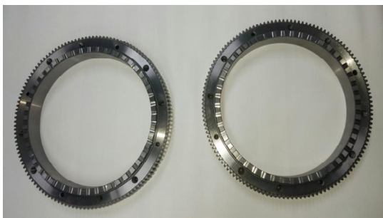
Fig. 4 Normal specimen and specimen with artificial defects
