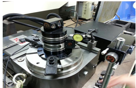
Fig. 3 Precision measuring instrument of reciprocating motion
