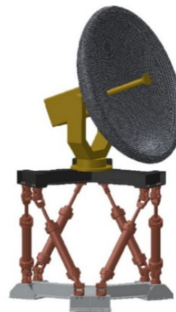
Fig. 2. Antenna on a six-axis motion simulator.
