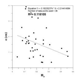
**Fig. 8.** Comparison of dispersivity with effective porosity for 36 long and short samples.
