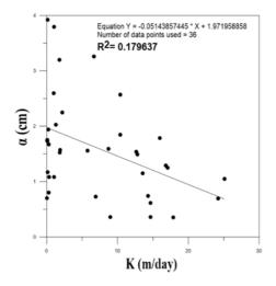
**Fig. 5.** Comparison of dispersivity with hydraulic conductivity for 36 long and short samples.
