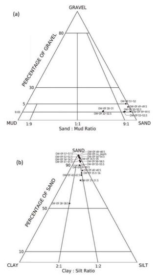
Fig. 3. Triangular classification (a) Gravel-Mud-Sand, (b) Sand-Clay-Silt of OW-9.
