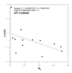
Fig. 10. Comparison of dispersivity with effective porosity for 13 short samples.
