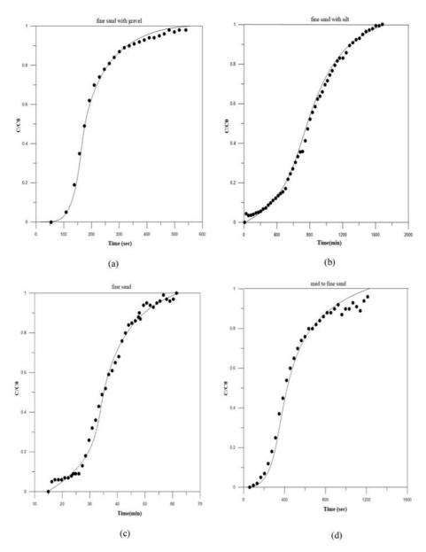
Fig. 4. Breakthrough curves of bromide solution for (a) OW-9 35.5 $\sim$ 36 m, (b) OW-9 51 $\sim$ 51.5 m, (c) OW-9 53 $\sim$ 53.5 m (d) OW-11 55 $\sim$ 56 m samples, respectively.
