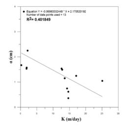
Fig. 7. Comparison of dispersivity with hydraulic conductivity for 13 short samples.
