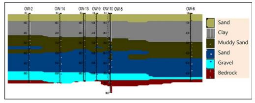
Fig. 2. Geological cross section of the study area.
