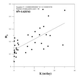
Fig. 11. Comparison of effective porosity with hydraulic conductivity for 36 long and short samples.
