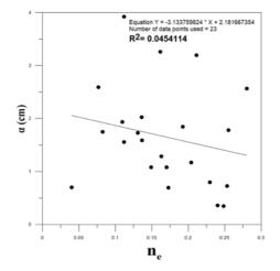
**Fig. 9.** Comparison of dispersivity with effective porosity for 23 long samples.
