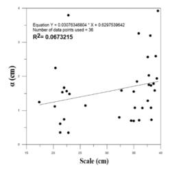
Fig. 12. Comparison of dispersivity with sample scale for 36 long and short samples.
