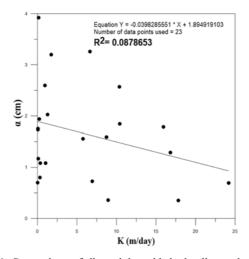
**Fig. 6.** Comparison of dispersivity with hydraulic conductivity for 23 long samples.
