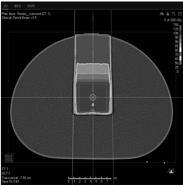
Fig. 5. Dose distribution when density override is used as the surrounding material of the gold fiducial marker.(The angle of gantry is 0 degree, the position of fiducial marker is 1 cm from the beam's end of the range.)
