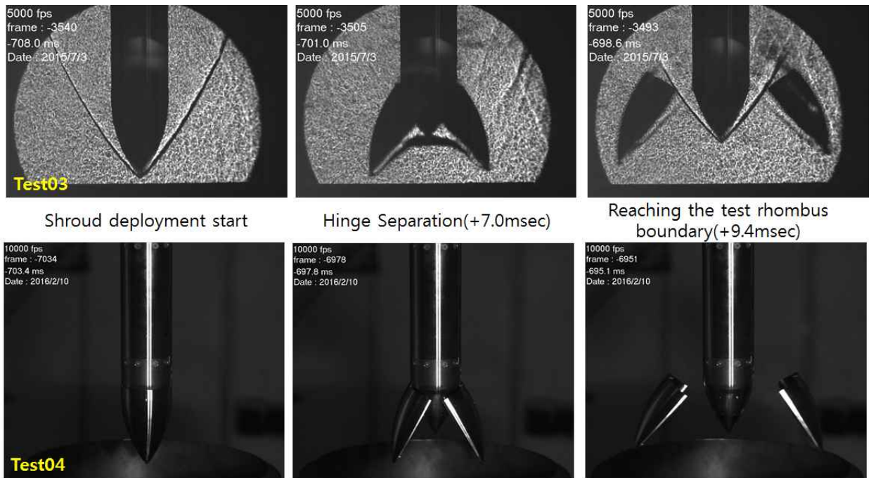
Fig. 13. Shroud separation behavior of Test03 and Test04
