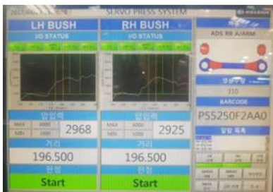
Fig. 13 Servomotor system in inserting bush
