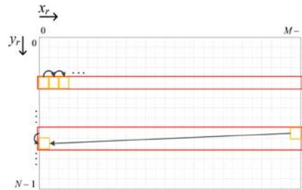
Fig. 2. Sequence of the pixel-unit calculation with a resolution of M \times N (adapted from [18])
