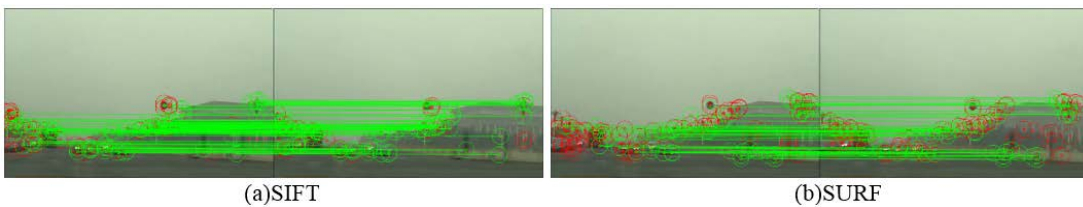
Fig. 9. The results of feature detection and matching for fuzzy images in Video 2 . The red circles represent single points or mismatch correspondences, while green circles and lines are correct matching points. The number of keypoints in this group tests is around 76.
