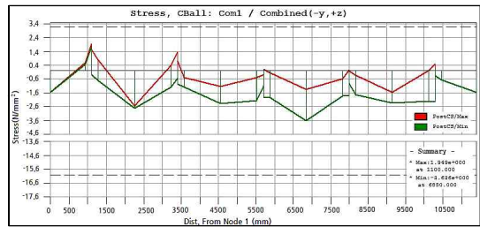
Fig. 14. Stress check of post-tensioned upper slab
