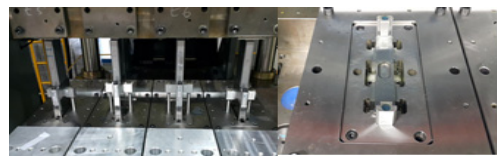
Fig. 4. Forging die for air vent manufacturing
