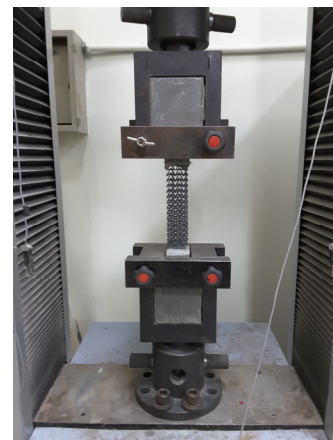
Fig. 8. Direct tensile test of auxetic mesh
