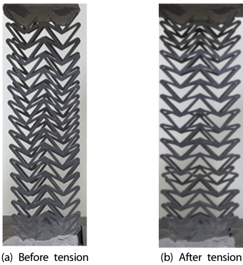
Fig. 10. Auxetic behavior of double arrow mesh( \theta_2=37.5^\circ )
