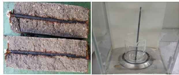
(a) Mortar after corrosion (b) Corrosion measurement
