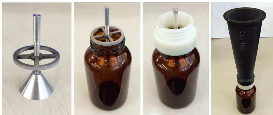
Fig. 2. Photographs of the circular cone attachment (diameter ( \varphi ) 36-mm for the conical bottom and 70^\circ for the vertical angle) for the cyclone.
