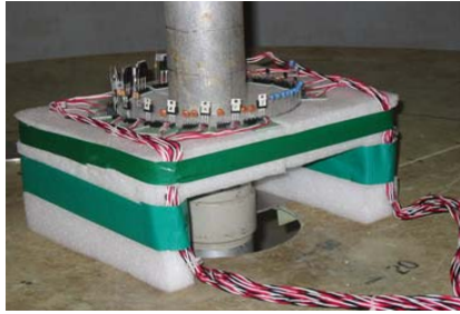
Fig. 5. The \gamma facility at KAERI for testing OP-Amp. and MOSFET.
