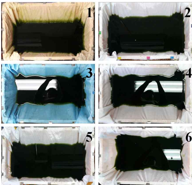
Figure 1. Shape of gravity-filtration devices using various membranes (1. CF1, 2. PE1, 3. PE2, 4. PE3, 5. PE4, 6. PE5).
