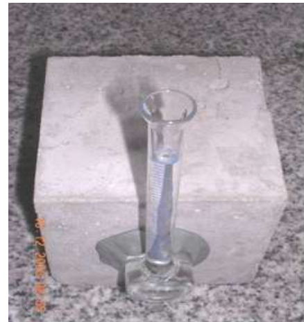
Fig. 5 Karsten flask on side face of concrete.
