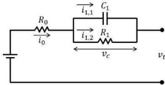
[Fig. 2] One ladder battery ECM
