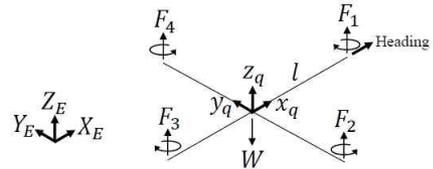
[Fig. 1] Quadrotor configuration
