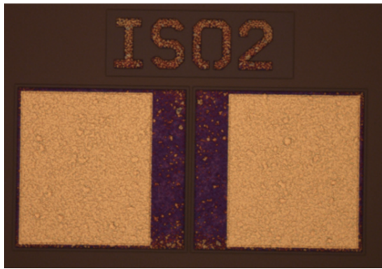
Fig. 1. Picture of buffer leakage test structure.
