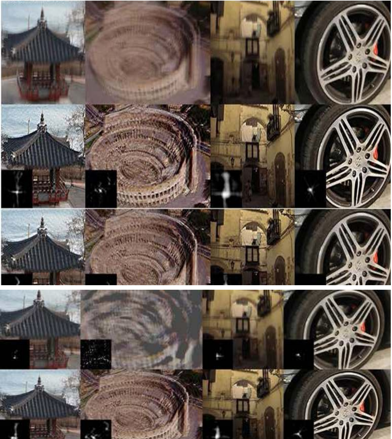
Fig. 13. Simulation results. [First row: original blurry images, Second row: Krishnan's method, Third row: Xu's method, Fourth row: Fergus's method, Fifth row: Our method], [First column: summerhouse, image_size: 800x795, kernel_size: 51x51], [Second column: roma, image_size: 800x533, kernel_size: 85x85], [Third column: street, image_size: 800x800, kernel_size: 65x65], [Fourth column: wheel, image_size: 800x533, kernel_size: 35x35].
