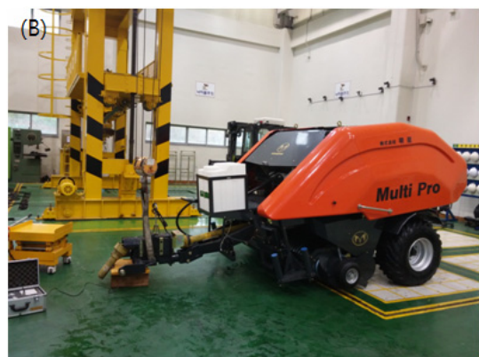
Figure 4. Measurement of the center of gravity in horizontal state and tilted state - (A): Tractor and (B): Baler.
