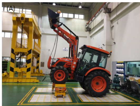
Figure 4. Measurement of the center of gravity in horizontal state and tilted state - (A): Tractor and (B): Baler.
