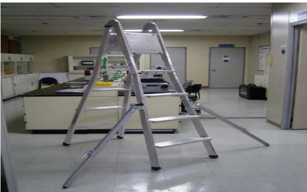
[Figure 5] Staircase safety ladder
