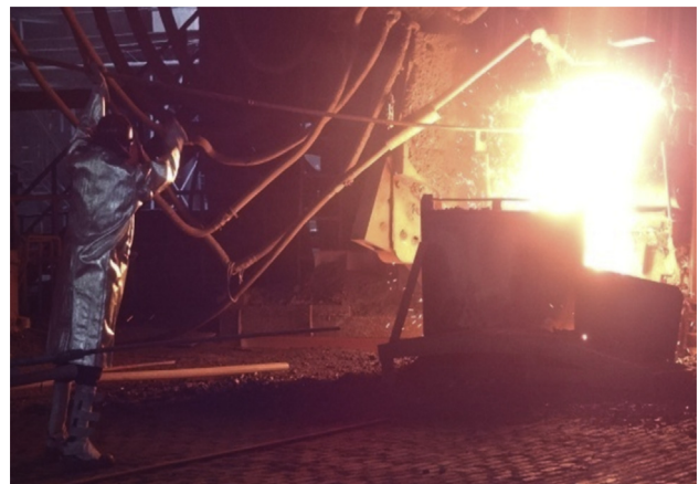
Fig. 1. Worker wearing aluminum overall exposed to radiant heat from furnace.
