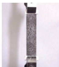
Fig. 8. Stretch the substrate specimen with both ends clamped.
