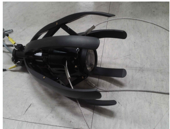
Fig. 2 Mechanism for measuring a diameter
