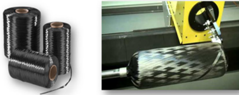
Fig. 2 Picture of tow prepreg and dry filament winding process [TCR Composites].
