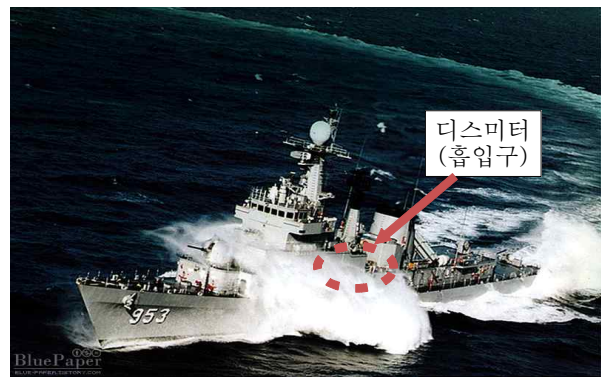
Fig. 7 Frigate in Operation at Sea(Saline inflow)
