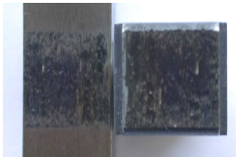
Fig. 1 Worn Ti-6Al-4V surfaces due to fretting: a flat Specimen (left) and a counterpart (right) [4]
