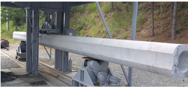
Fig. 9. Bending moment test of PHC-W pile
