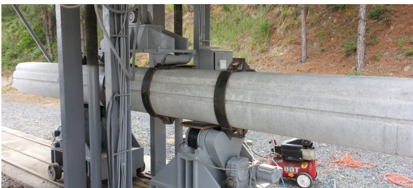
Fig. 10. Shear strength test of PHC-W pile
