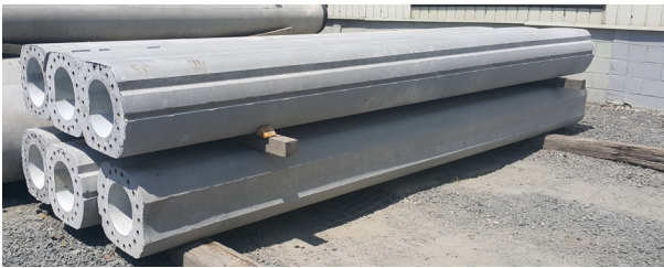
Fig. 6. Produced PHC-W piles
